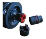
There is a set of soft coupling between electric motor and air end for efficient power transmission of driving. The coupling is reliable, and has the function of smooth connection of motor axis and air end axis, and reduces the shock load caused by starting torque.
